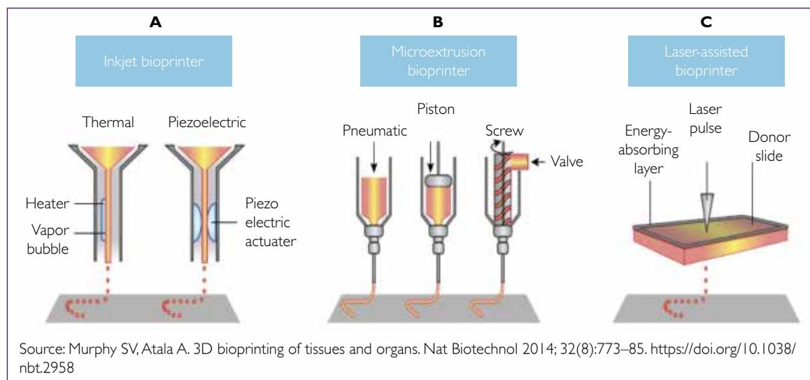
Figure 16: Schematic components of inkjet, extrusion and laser-assisted bioprinters<sup>277</sup>
